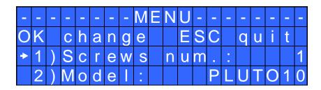
1) Screws number: EDU2AE/HPRP/TA can act as screw counter. You can set the number of screws from 1 to 99. To disable the function select OFF by pressing  $\mathbb{Q}$  as many times as needed.
