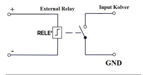
As for the outputs, they are all PNP type with active function. On each pin you will have 24V DC.
