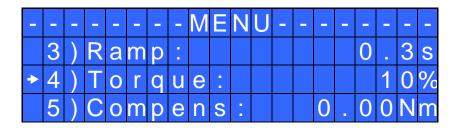
**3) Ramp:** You can select the slow start time (acceleration) from 0.2 to 3.0 sec. This option is only available for the screwing phase, while during the unscrewing phase the ramp time is always 0.2 sec. We suggest using this option with self-tapping screws.
