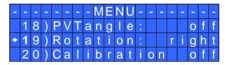
**18) PVTangle** – **Prevaling Angle Torque:** it indicates the angle that the screwdriver must reach at the maximum torque and then continue at the pre-set torque. The angle can only be set if the "TORQUE/LEVER" mode (23) is active, therefore when the lever is pressed, the screwdriver will turn at maximum torque.
