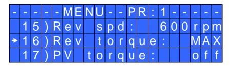
**15) Rev speed** – **Reverse speed**: You can select any reverse speed value of the screwdriver between the maximum and the minimum specific speed of every single screwdriver (see table with technical data).
